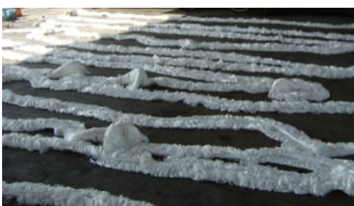
Photo 3 Braided adsorption material combining adsorption function and mooring function
