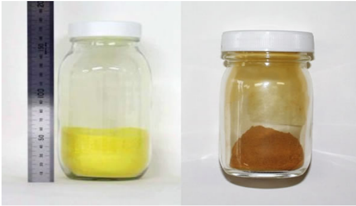
Photo 2 Uranium (left) and vanadium (right) collected from the ocean
